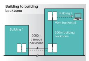
It is important to note that these maximums apply to all media. They do not take into account the performance differences between cable types and transmission **protocols** used by the network. In practice, maximum cable lengths will depend on the **application**, the type of network used (e.g. **1000BASE-T**) and the cable's quality. Good cable suppliers and installers will advise on a **cabling** system's capabilities in a particular network.
