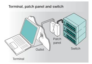
CENELEC EN50174 and TIA/EIA 569 cover many aspects of outlet location for mounting in walls, floors and furniture. In addition to standards criteria, accessibility must be considered.
