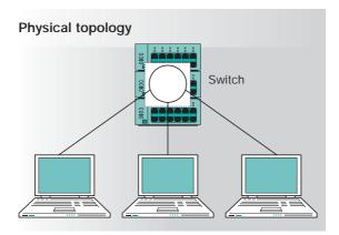
An example of this can be seen in the diagram above. The system shown has the appearance of a star, but its logical topology remains a true ring, with the loop completed within the central switch. Networks based on star, bus and ring type logical topologies all have their advocates, and the final choice largely depends on the application. The star physical topology, however, is now almost universally accepted within commerce and industry.
