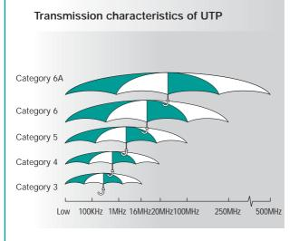
For new installations, Category 6A or Class  $E_A$  cabling guarantees 10GBASE-T support to 100 m over UTP. Since the international Class  $E_A$  specification is more stringent, cabling for new installations intended to support 10GBASE-T should be specified to meet the Class  $E_A$  requirements.
